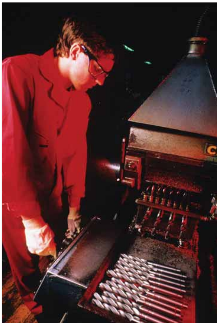
Flute milling of taper shank drills
