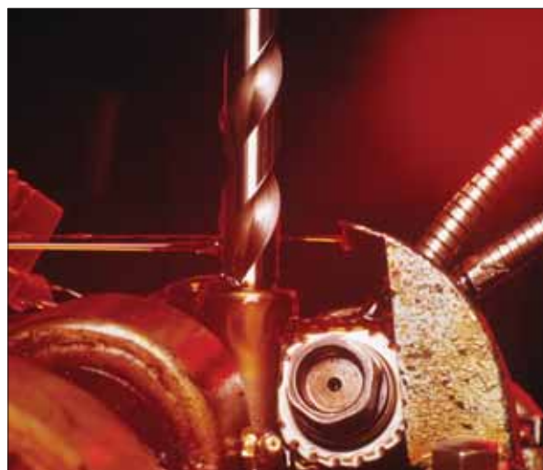
Flute milling of large diameter twist drills
