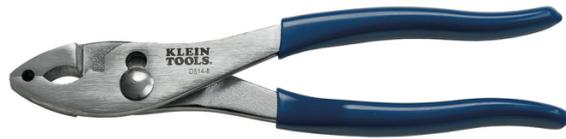
Use Klein Tools' 8-Inch Hose Clamp Slip-Joint Pliers to quickly install and remove spring-tension hose clamps. These pliers grip with either end or side of jaws. Designed for work in confined spaces.
