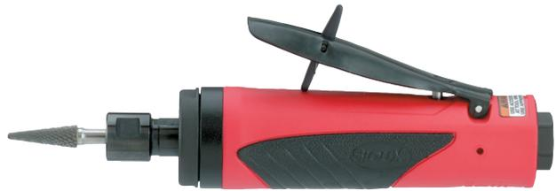
Over speeding wheels can explode. Check the speed rating of the accessory or the speed printed on the wheel. This speed must be greater than the name plate speed of the grinder/sander and the actual speed of the grinder/sander as measured with a tachometer.
