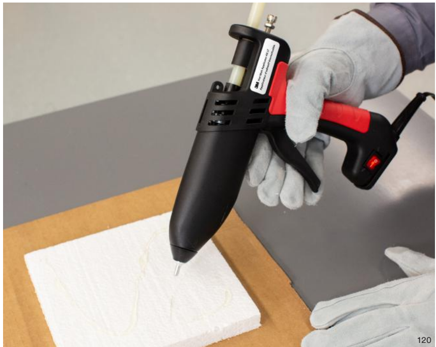
3M™ Hot Melt Applicator LT with 3M™ Hot Melt Adhesive 3762LM low temperature (265°F/129°C) adhesive effectively bonds heat-sensitive substrates such as styrene foam to itself, corrugated or other surfaces without damaging the foam.
