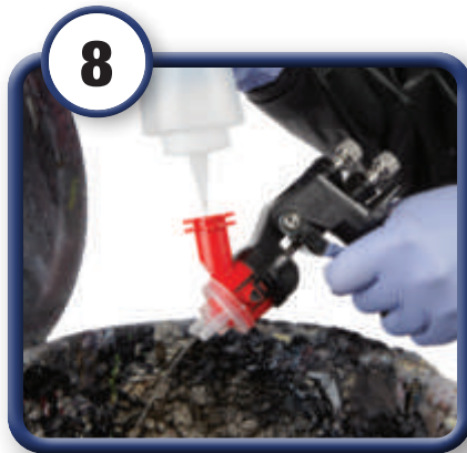
8 Flush out atomizing head with appropriate solvent until the atomizing head is clear of coating.
