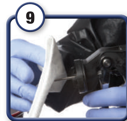
9 Wipe off any additional residue from the fluid needle.
