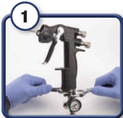
1 Hand tighten or use two wrenches to connect the air flow control valve.
