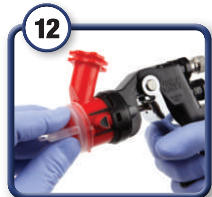
12 Re-attach the same atomizing head or when necessary replace with a new one.
