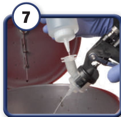
7 Flush out atomizing head with appropriate solvent until the atomizing head is clear of coating.
