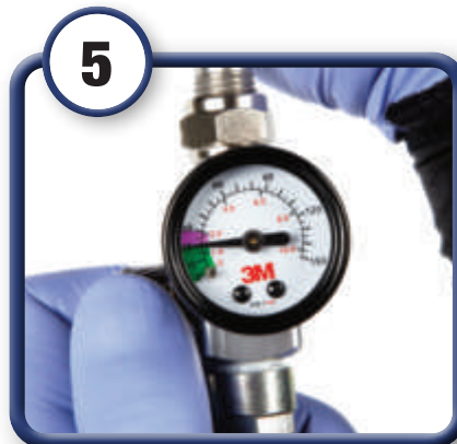
5 Set air pressure at 15 psi for 2 nd stage (air and fluid flowing)
