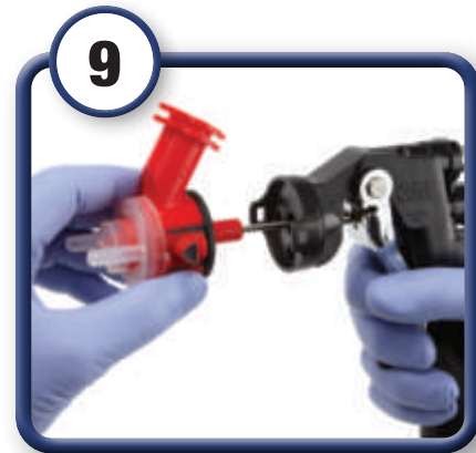
9 Remove atomizing head - be sure to pull trigger back and pull the atomizing head straight out from the gun body to avoid bending the fluid needle.
