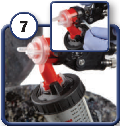
7 When you are finished using the system, pull the trigger back to release fluid back into cup, remove the air line, and the 3M™ PPS™ Cup.
