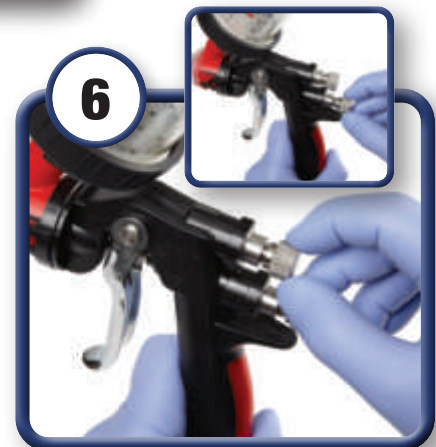
6 Adjust fan and fluid flow to achieve the desired size and wetness of the pattern. NOTE: when closing the fan adjustment completely it may be necessary to re-adjust the air flow control valve.
