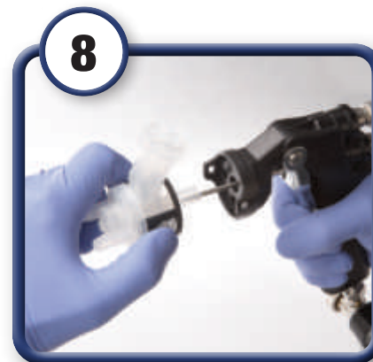
8 Remove atomizing head - be sure to pull trigger back and pull the atomizing head straight out from the gun body to avoid bending the fluid needle.
