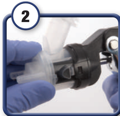
2 Attach an atomizing head to the gun - pull trigger back and hold, making sure the release buttons are aligned with latch openings - listen for a double click to ensure that it is fully engaged.
