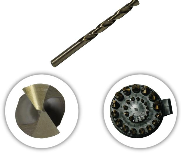
135 Degree Split Point for Self-Centering and Reducing Thrust
