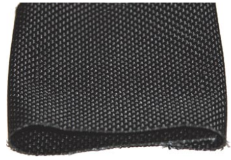
Ballistic Nylon (BN) 1/16" Thick
