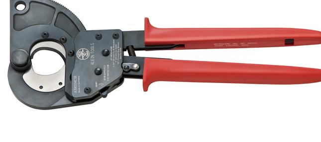
These Klein Tools ACSR Ratcheting Cable Cutters are equipped to cut up to 477 MCM ACSR multi-strand. They have high-leverage ratcheting mechanisms for easier cutting, and can be locked when not in use. They are size efficient as well, with a length just under 14-Inches they can be carried around in a tool pouch.
