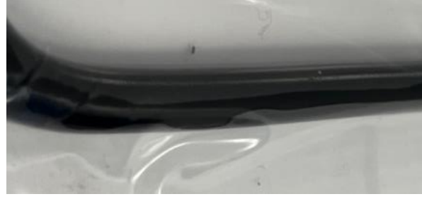
Figures 1-2: Tight liner adhesion on left, premature de-bonding due to low liner adhesion on right
